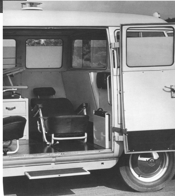
On the right: an inside view of a Miesen ambulance. The rotary fan on the roof is visible and there is no air intake. You can also note the side step, which slides in a sill extension. [3]
