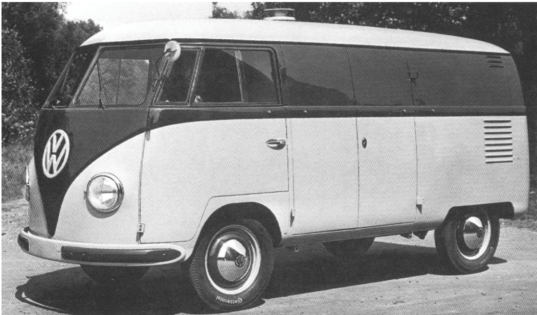
A very nice Transporter with the M55 rotary fan. This one has the 175 mm long louvers. Type is 213 or 215. Also note lockable cargo doors. [1]
